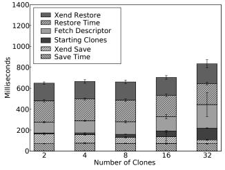
Figure 3: Fast Clone Creation. Legend order matches bar stacking from top to bottom.
