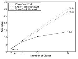
(c) Multicast Scales. BLAST, 256MB DB. Speedup vs. one thread, labels show absolute times.
