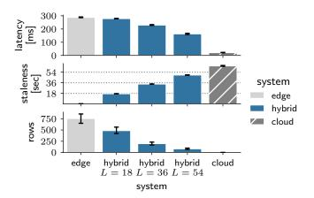
Fig. 7. Mean query latency, result staleness, and bandwidth (rows sent over the network) when running global queries on the medium topology using different global querying systems.
