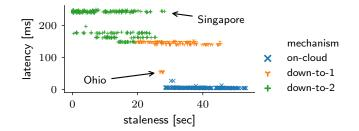
Fig. 14. Staleness vs latency of the answer for each query in the real-world experiment. For clarity, we only show a sample of the queries. The varied latency from cloud to the different nodes is reflected in the different latency-staleness clusters in the figure.
