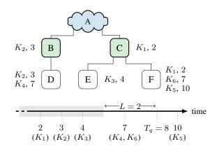
Fig. 3. Edge network with 6 rows  $K_1$  to  $K_6$ , with row update times (numbers next to keys). A query submitted to A at time  $T_q = 8$  with laxity of L = 2 must retrieve all keys updated before time  $T_q - L = 6$ , and must therefore access nodes B, C and E, but not D and F.
