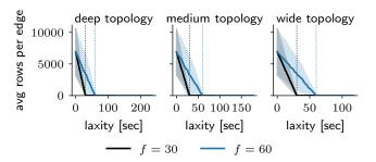
Fig. 11. Average number of rows accessed by each local edge replicas as a function of laxity for different with push period f = 30 seconds and f = 60 seconds. Feather shifts work from edges towards the core and cloud nodes, and once L > f edges are seldom involved in answering global queries. Shaded areas show standard deviation. Dotted vertical lines show push period f.
