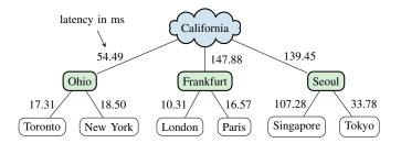
Fig. 13. Topology of the real-world experiment. Numbers indicate mean measured round trip time in milliseconds.
