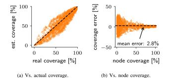
Fig. 12. Rows covered per query across all topologies and laxity ranges. (a) estimated row coverage compared to real row coverage. Dashed line shows equality (Y=X). (b) estimation error (the difference between estimate and real row coverage) as a function of how many nodes participated in the query. Dashed line shows the mean coverage estimation error. For clarity, we only show a sample of queries.
