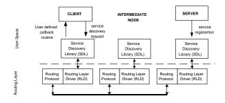
Fig. 1. Cross-Layer Service Discovery Architecture
