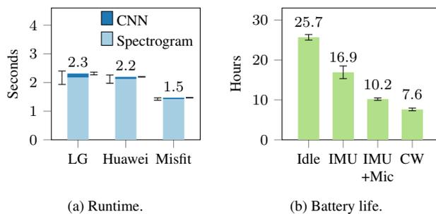
Fig. 6. Runtime of running our system on three smartwatches (a), and resulting battery life on LG Urbane under different operating modes (b). Error bars show standard deviation.
