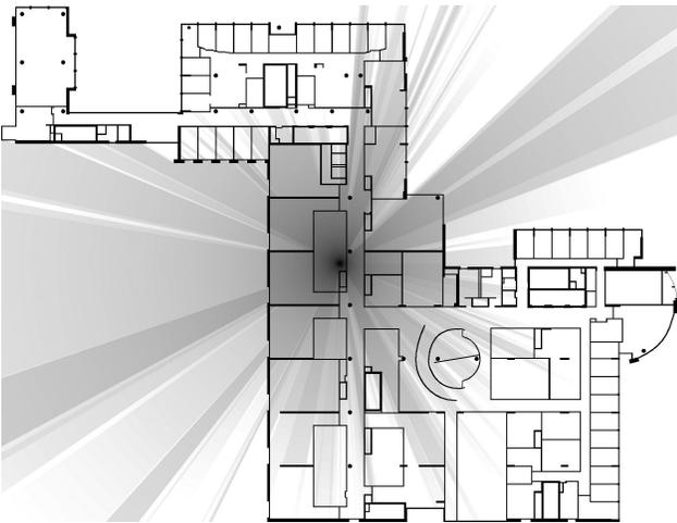
Fig. 3. AF generated visualization of signal strength.
