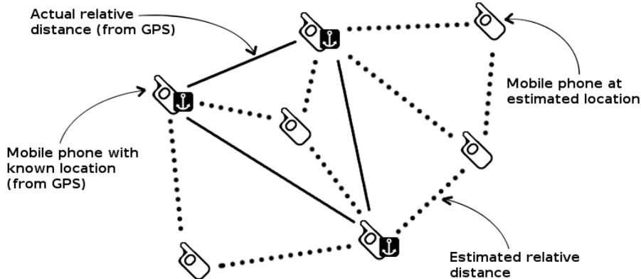
Fig. 1. Absolute positioning of mobile phones using Calibree.
